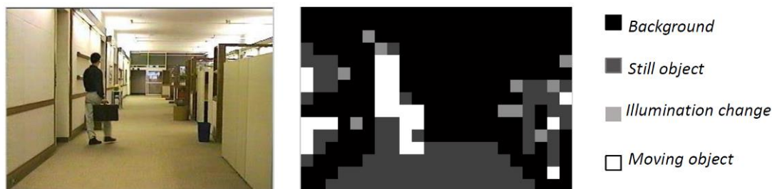
Figure 7. Example of Block classification output stage. Left: Image under analysis. Right: Image of each block labels: Background, Still object, Illumination change and Moving object.
