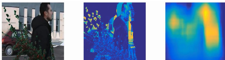
Figure 20. Example of non-precise motion information from LabGen-P. From left to right: Image, frame difference and motion information (spatially-expanded frame-difference). Note that this motion information does not accurately reflect the true image motion.
